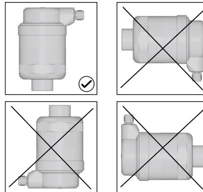
It is possible to rotate the air vent valve through 360°C to position the discharge appropriately without needing to shut down the system.
