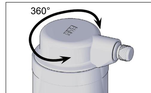
**WARNING!** Once you fill the system, it is advisable to close the air vent valve by turning the cap clockwise
